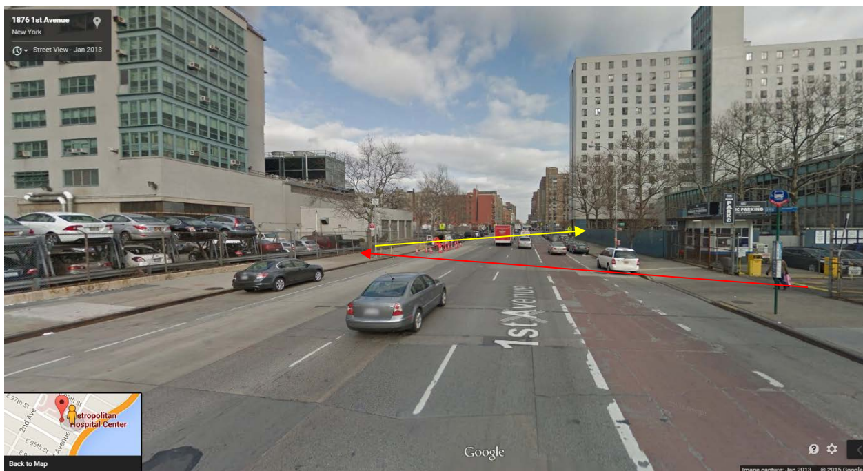
FIGURE 8. RED ARROW DEMONSTRATES WAVES APPROACHING FROM THE EAST RIVER AND IMPACTING THE EXISTING METROPOLITAN HOSPITAL BUILDING FACE OR PROPOSED WALL. YELLOW ARROWS SHOW WAVE REFLECTION PATHWAYS TO THE WALL EXTERIOR TO DRAPER HALL, EAST OF FIRST AVENUE.
