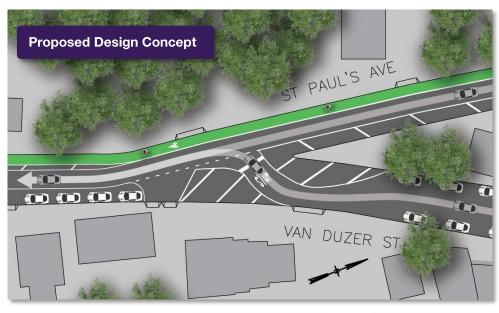
Improve Visibility Reorient intersection improves visibility and adds parking Standard Travel Lane Widths Discourage speeding with standard travel lane widths Clear Up Traffic Signs Allows for better placement of signs
