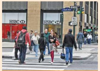
A 10 ft wide refuge island was installed on the south side of E. 33<sup>rd</sup> Street at Park Avenue to provide safer environment for pedestrians.
