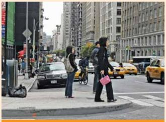
The curb extension on the southeast corner shortens the crossing distances and aligns the curbs to make for a safer crossing.
