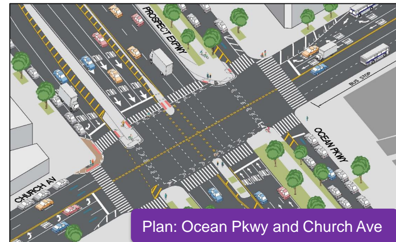
Expanded concrete median, NW service road
