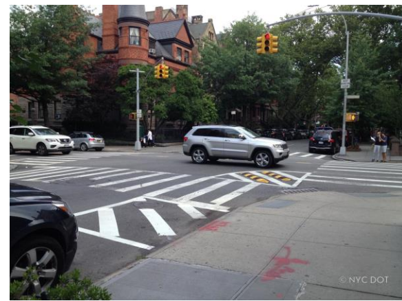
Photo: Proposed condition of right turn traffic calming at Union St and 8 th Ave
