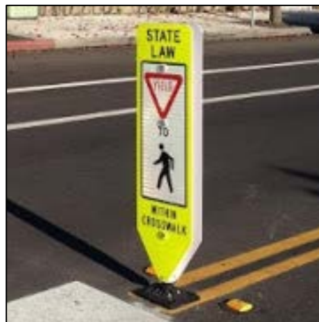
In-road Paddle Sign (currently in pilot testing)
