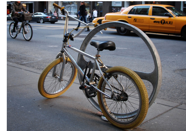
NYC DOT CityRack Dimension: 33.7" diameter Cast Metal
