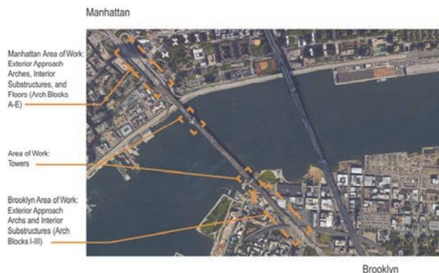
The Manhattan Approach is a continuous arch masonry structure consisting of brick, granite, limestone and infill concrete. The arches run between the Manhattan Anchorage at the east and
