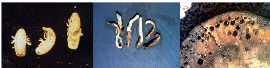
Marine Borer – Limnoria Species. Marine Borer – Teredo Species. Teredo Damage (Holes up to ¼" Diameter).
