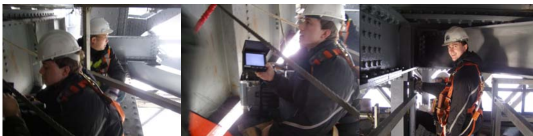
The Consultants Used the Division's Borescope on the Williamsburg Bridge to Inspect Fracture-Critical Details That They Were Unable to Access by Their Own Devices. They Were Assisted by Mechanical Engineering Intern Anton Depasquale. (Credit: Kevin McNulty)
