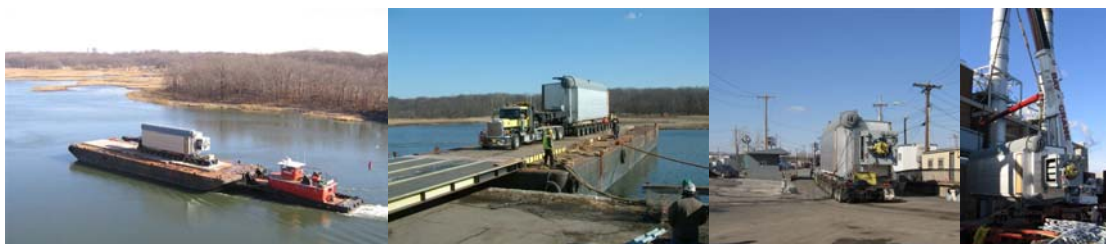
In February 2007, a Permit Was Issued for the Move of a Boiler to Co-op City in the Bronx. The Boiler was Unloaded From a Barge at the Agency Conner Street Facility, and Was Later Delivered by Truck to Its Final Destination. The Total Weight of the Vehicle With the Boiler was Approximately 380,000 Pounds.
