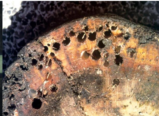
Teredo Damage (holes up to 1/4" diameter)
