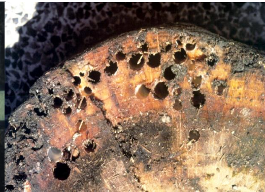
Teredo Damage (holes up to 1/4" diameter)
