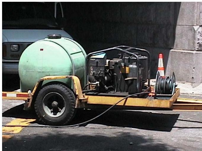
Pressure Washing Machine Used for Graffiti Removal.
