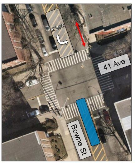
Concrete pedestrian safety island and left turn bay will require minor parking removal to accommodate emergency vehicles
