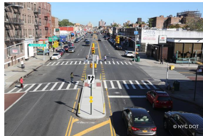
Proposed condition (pedestrian island) for Ocean Parkway and Avenue X (Photo: Hillside Ave and Sutphin Blvd)
