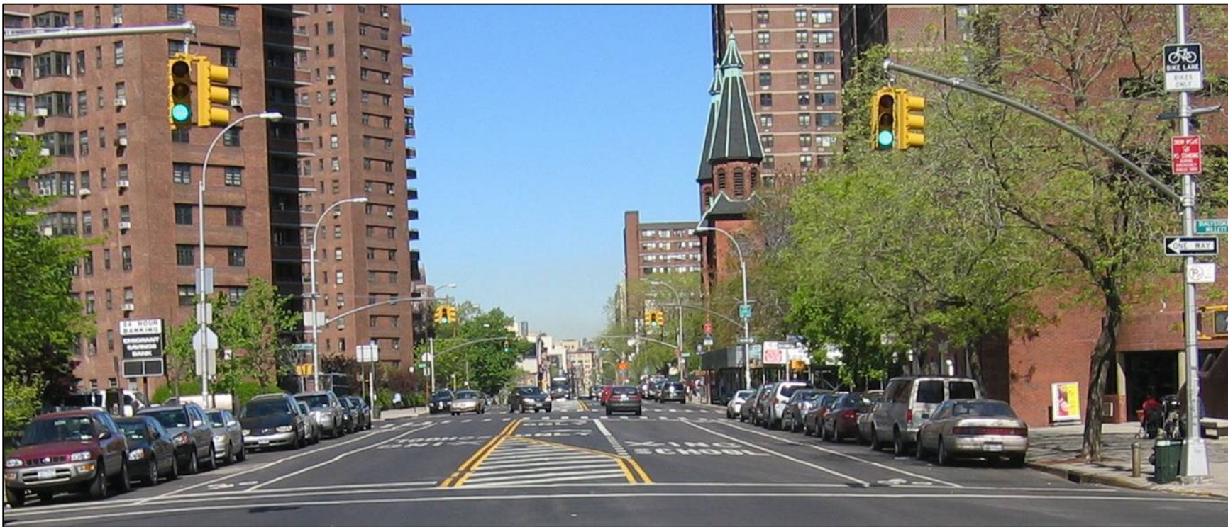
Grand Street, Manhattan: 2-way street with Bicycle Lane, a Moving Lane, Turning Lanes and Center Painted Median
