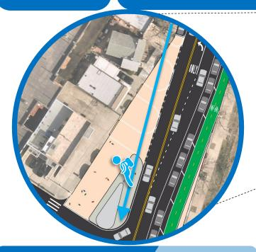
Expand existing concrete island and provide direct and safe pedestrian path
