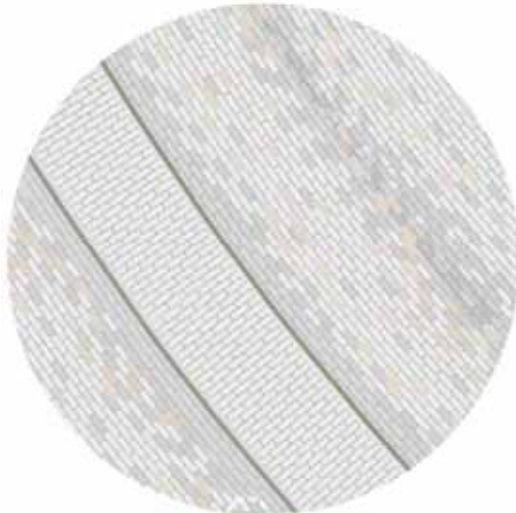
RAIL LINE PAVING DETAIL: HORIZONTAL COBBLE 12"X 4" LIGHT GREY
