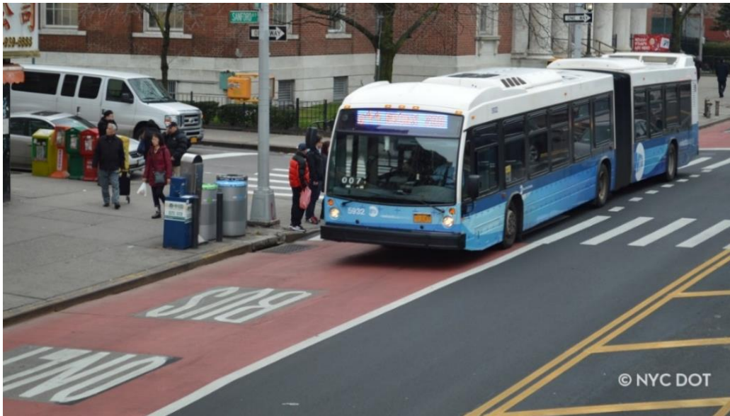
Example of curbside bus lane
