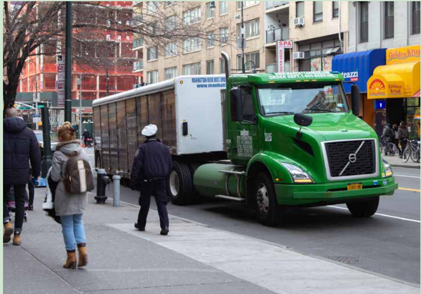
Typical truck cab designs can obstruct a driver's view of pedestrians
