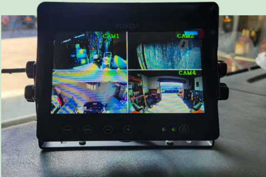
Camera technology can help compensate for obstructed vision
