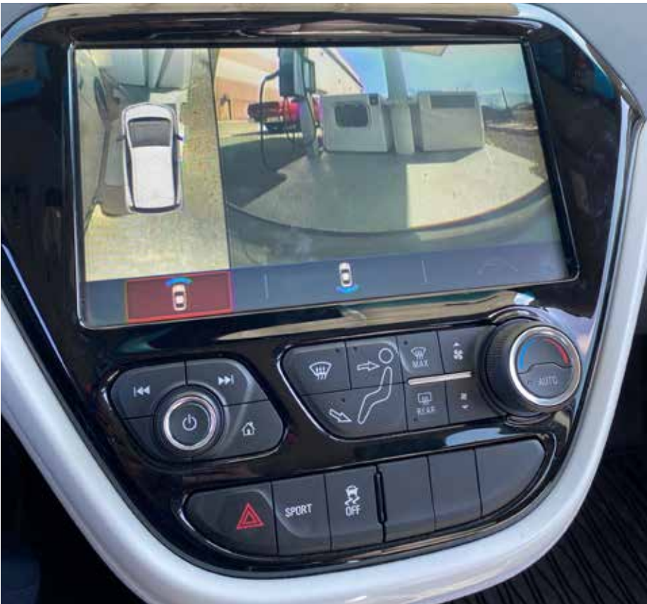
Surround cameras can compensate for obstructions to direct vision
