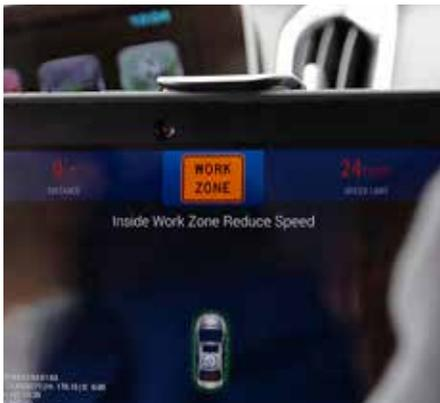
Connected Vehicle Technology allows vehicles and infrastructure to electronically "communicate".
