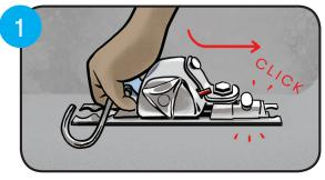
Slide front securement into tracks.
