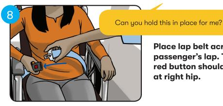
Place lap belt across passenger's lap. The red button should be at right hip.
