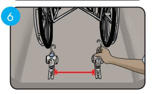
Slide back securements into tracks.
