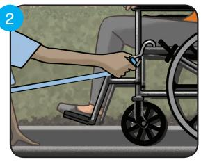
Attach hook to securement spot.
