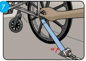
**Hook straps onto** back of wheelchair and tighten.
