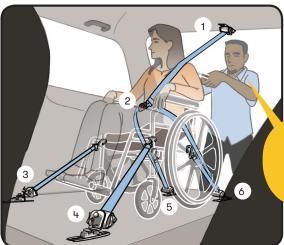
Test the securements gently push and pull the wheelchair to make sure the securements keep the passenger in place.
