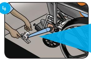
Tighten front securements.
