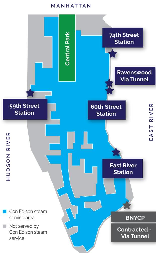
*This figure shows the Con Edison steam system service territory. The blue stars indicate the locations of central steam generation plants that are owned and operated by Con Edison. The gray star indicates the cogeneration plant in Brooklyn that is not owned and operated by Con Edison but delivers steam to their steam system in Manhattan according to a contract between both parties.*
