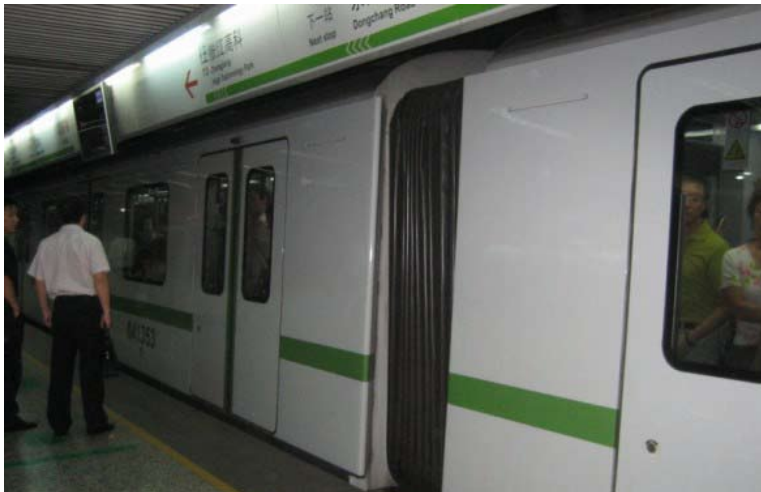
The exterior of one of Shanghai's internal gangway subway cars. Similar to an elongated bus, the moving gangway between subway cars is protected by a flexible "accordion" casing allowing passengers can travel freely throughout the length of the train. NYC Dept. City Planning
