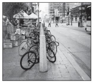
Secure bike parking in Minneapolis where a metal ring attached mid-way to a post allows the frame and one wheel of the bicycle to be locked on, - an effective way of using existing street furniture for bicycle parking.
