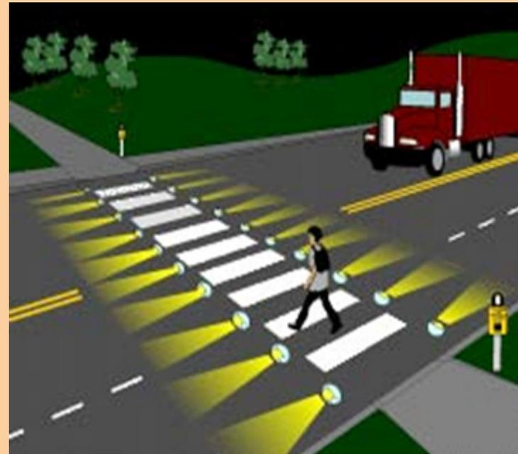
IMAGE 13. The schematic shows how the flashers work. As a pedestrian enters the crosswalk, flashing LEDs embedded into the pavement start flashing to warn drivers. Image used with permission from the Pedestrian and Bicycle Information Center.
