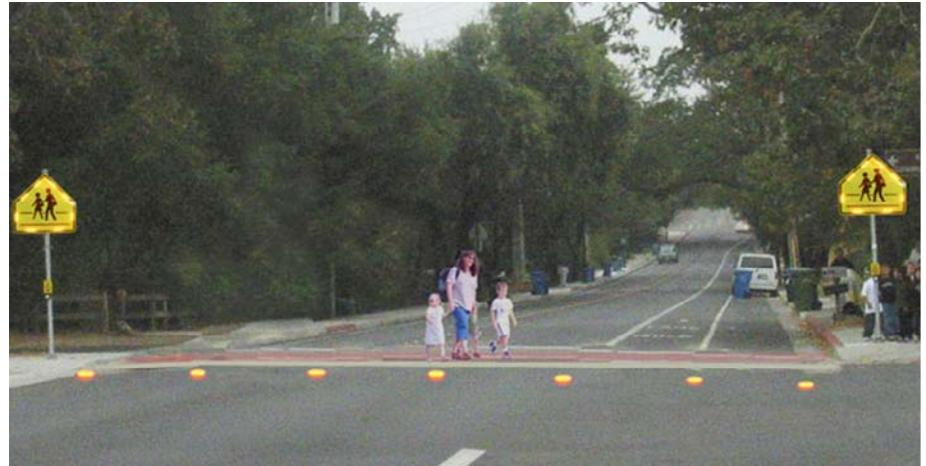
IMAGE 15. *Embedded Flashers-The LED flash after the pedestrian enters the crosswalk. Image used with permission from Lightguard Systems, Inc.*
