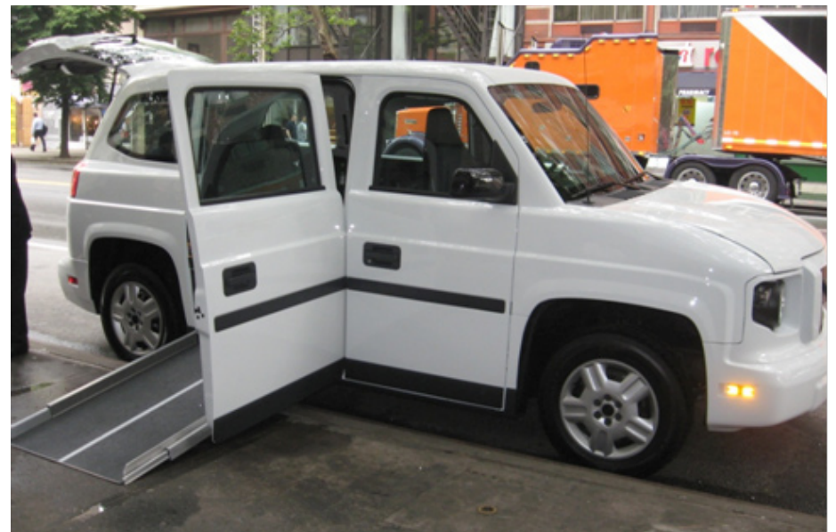
IMAGE 11. MV-1 with ramp shown with ramp extended for wheelchair access. NYC DCP.
