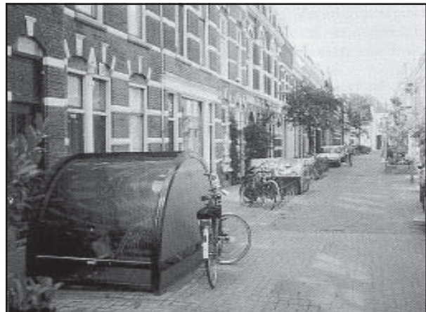
The Bicycle Drum is an innovation for older neighborhoods where houses often lack enough storage space (source: Moderne Rad-verkehrsanlagen und Fahrrad-Infrastructure-Perspektiven fuer Muenchen ).
