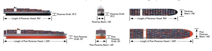
Figure 4: Comparison of Panamax and Post-Panamax Container Vessels
