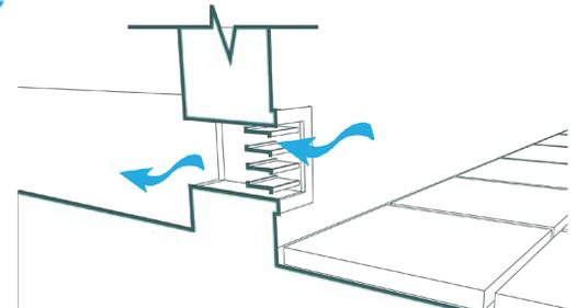
When wet floodproofing, openings for water penetration and exit must be engineered according to ASCE 24 requirements. A minimum of two openings is required for each enclosed area below the DFE, to be installed on at least two sides of each enclosed area. The opening should be located no higher than 1 foot above the grade immediately under each opening.
