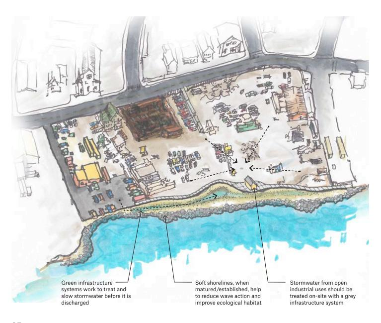
Unenclosed and unsecured inventory vulnerable to flooding: Auto parts and valuable salvaged materials that are submerged due to flooding, especially with saltwater, are likely to develop rust or be destroyed, eliminating their resale value. In addition to damaged inventory, unsecured auto parts and scrap metal that are dislodged by flooding can severely harm structures or equipment on the property and create similar hazards for nearby properties.
