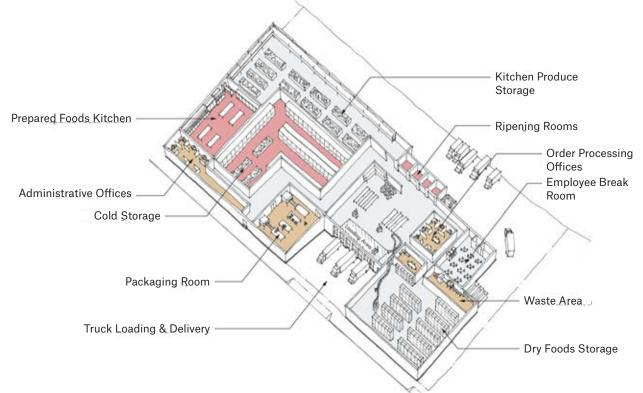
**Ripening rooms, cold storage and the prepared foods kitchen have significant investments in equipment:** Ripening rooms are key components of the distributor's operation and tend to contain more investments in equipment that could be damaged by floodwaters. While it may not be cost-effective for the business to fully protect the entire facility, the potential for flooding within key areas of the building that contain more sophisticated equipment is a significant risk.
