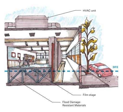
Film-making equipment highly vulnerable to flood damage: Cameras, microphones, lights, stands, cables, and other equipment are often stored at grade within production studios so they can be easily accessed and used. Without storage space above the DFE, this equipment is likely to be inundated during flood events. Damage to these assets not only results in high replacement or repair costs, but can also hinder operations and delay production.
