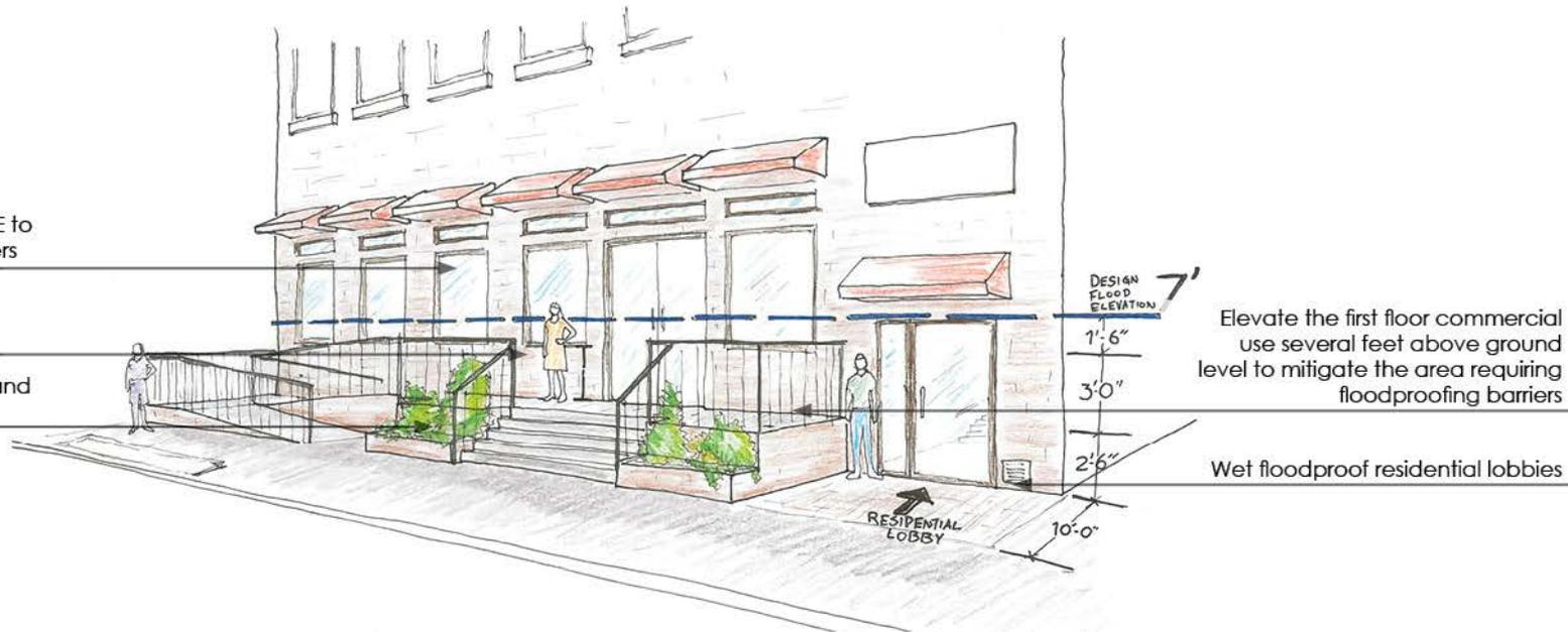
Elevate the first floor commercial use several feet above ground level to mitigate the area requiring floodproofing barriers
