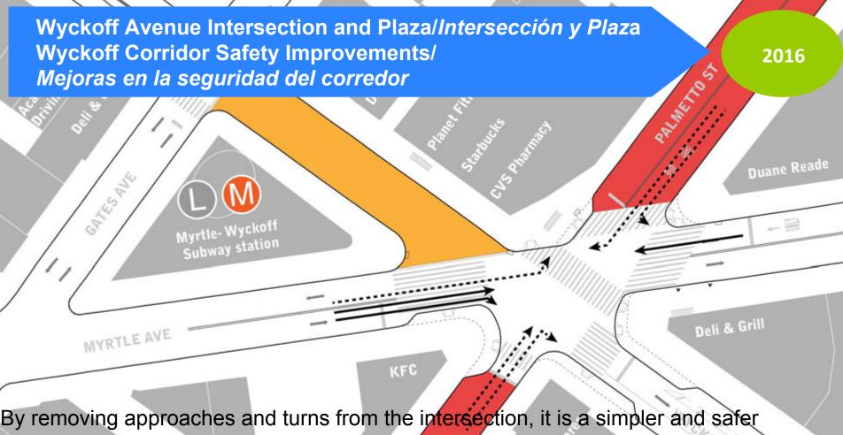
By removing approaches and turns from the intersection, it is a simpler and safer place
