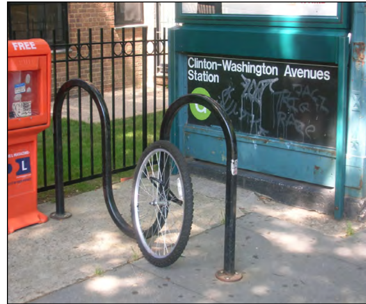
Square tube wave rack. Improperly locked bicycle at only one point of the bicycle is an opportunity for a bike thief.
