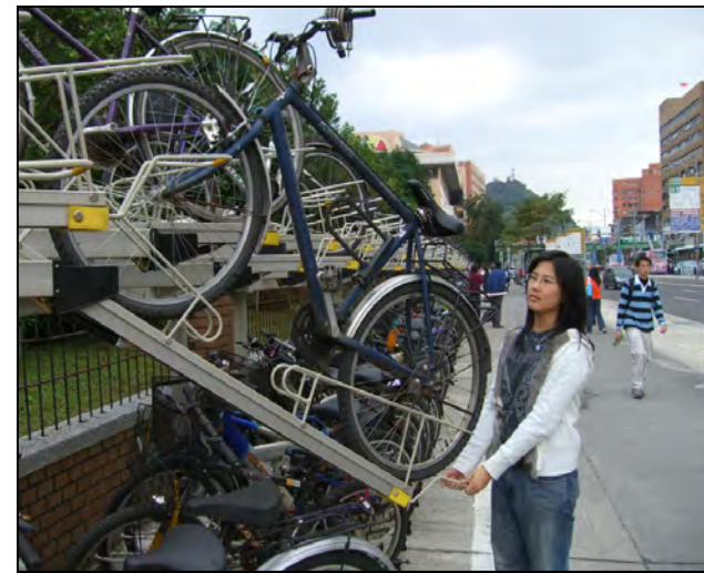
Right: A 2-Tiered hydraulic bicycle rack at a transit station in Taipei, China: www.trtc.com.tw
