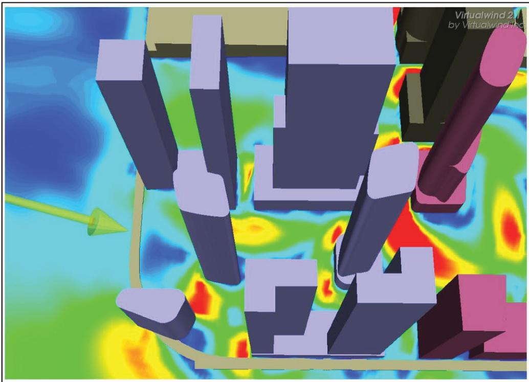
Wind Simulation Results: Full-Build Configuration
