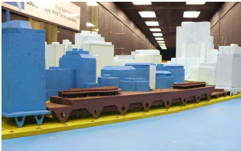
Figure 11: Wind Tunnel Test Model Views from South
