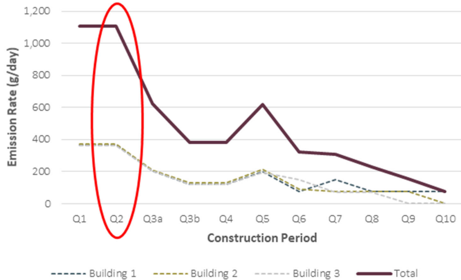
Figure 11-3: Short Term (24-hour) PM 2.5 Construction Emission Profile
