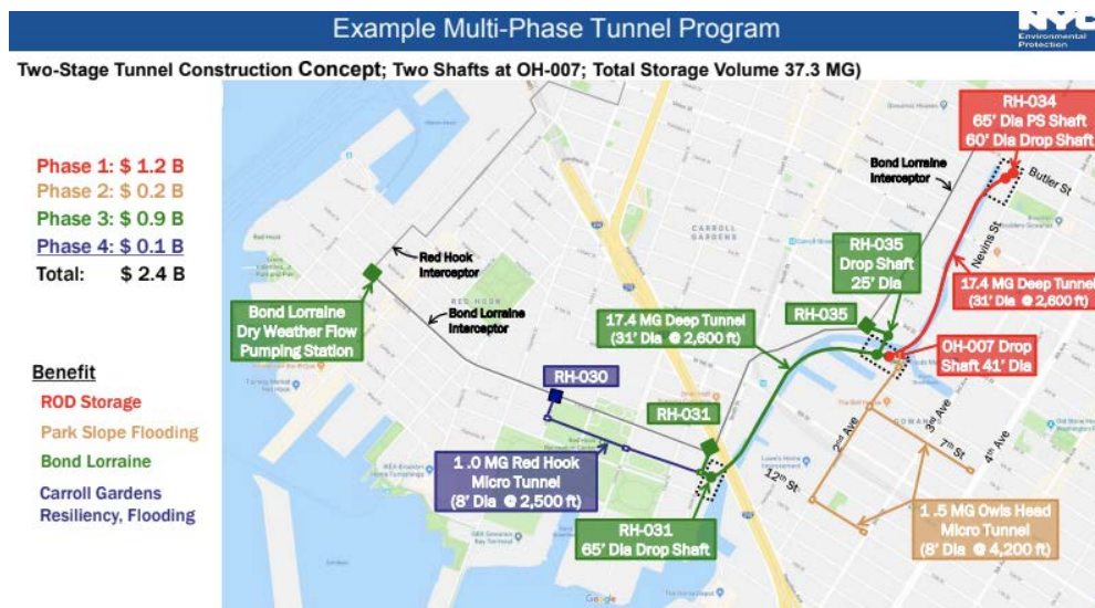
Figure 11-3: Proposed Infrastructure Upgrades at the Bond-Lorraine Sewer 37
