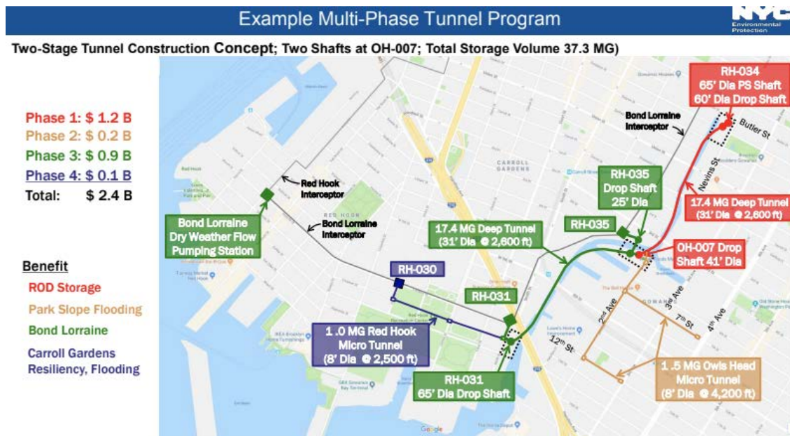
Figure 11-3: Proposed Infrastructure Upgrades at the Bond-Lorraine Sewer 60
