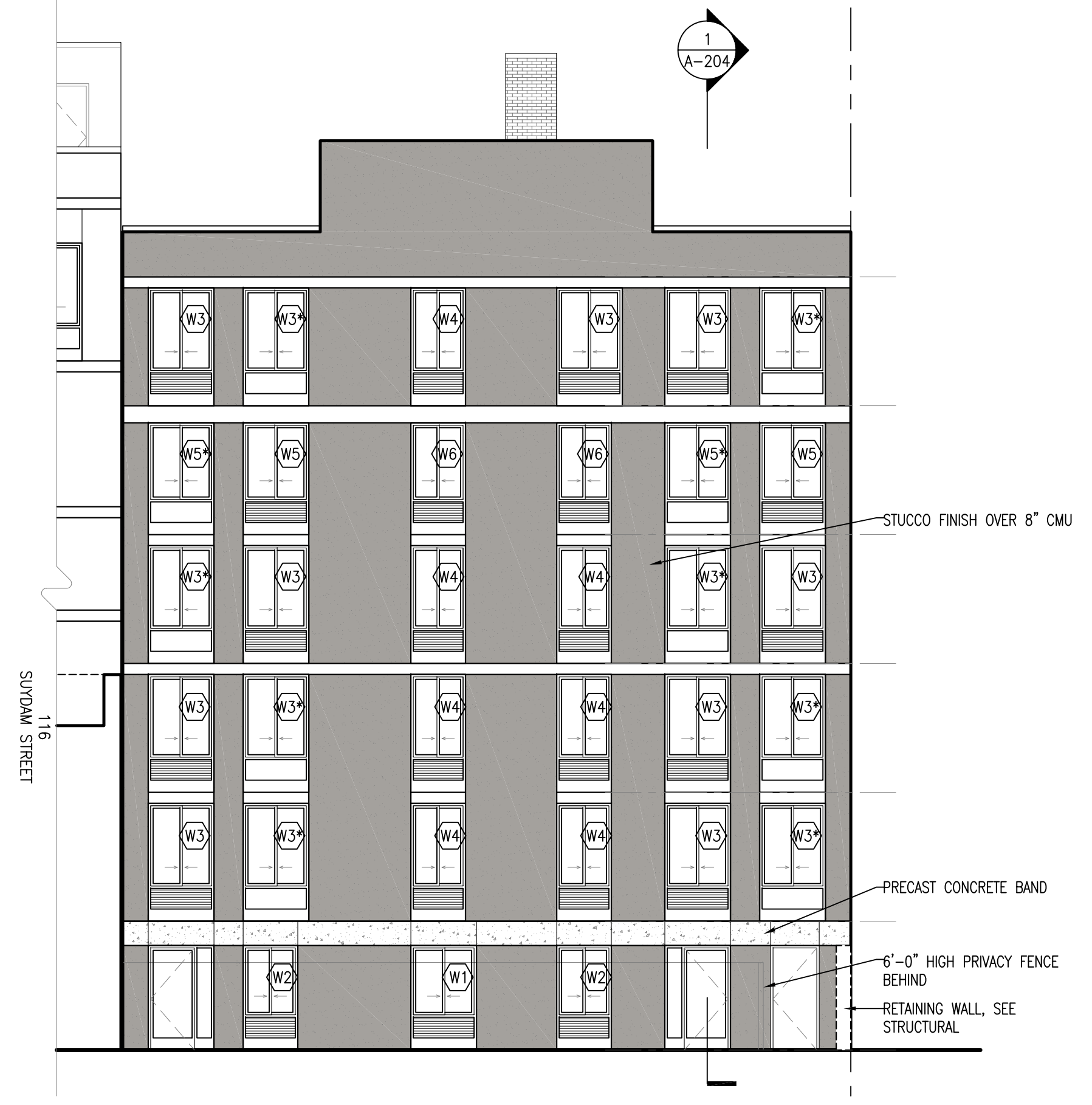
2 SOUTH ELEVATION-118 SUYDAM STREET 1/8" = 1'-0"
