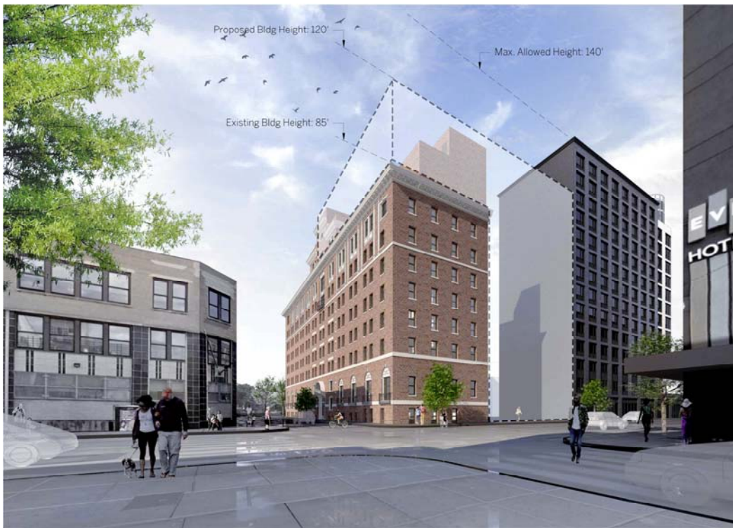
Figure UD-2: Existing Building, and Massing for Proposed With-Action Condition View from Northeast
