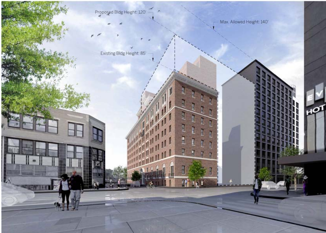
Figure Residential 1: Existing Building, and Massing for Proposed With-Action Condition and Height Limit, View from Northeast
