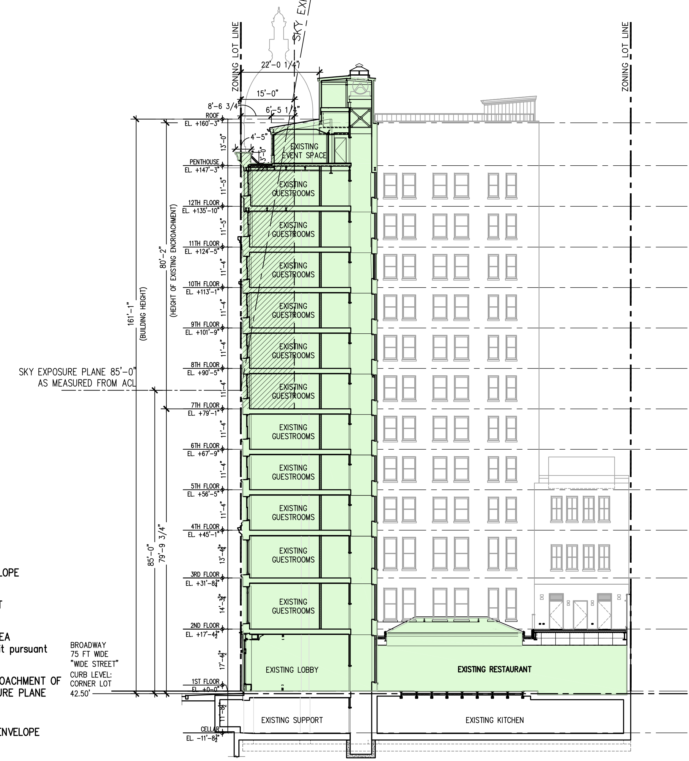
1 EAST-WEST SECTION - 1170 BROADWAY SCALE: 1/16" = 1'-0"
