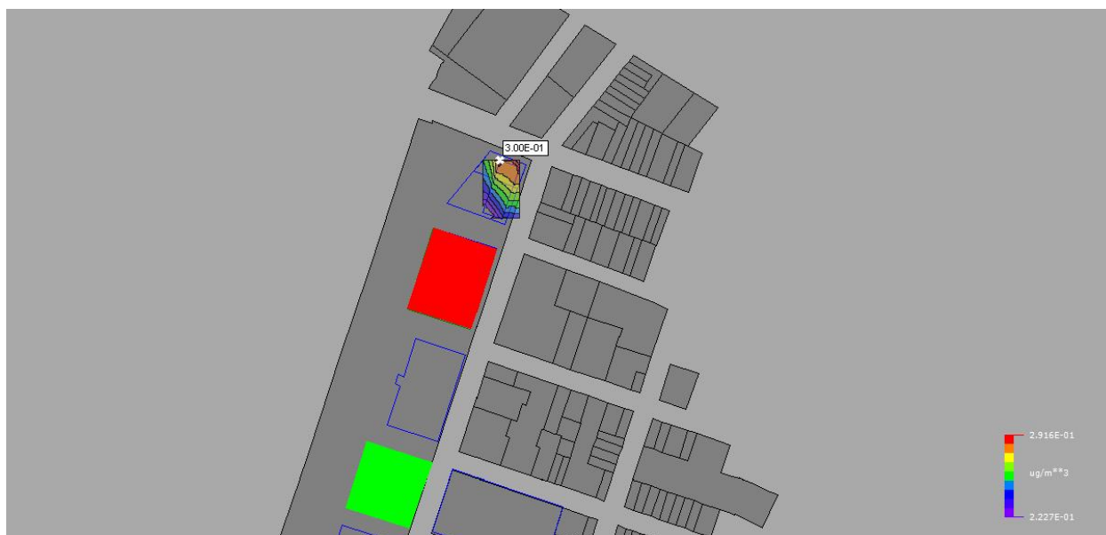
Figure 3: The Max Estimated 24-hour PM 2.5 Impact at 50 feet Windows Receptors
