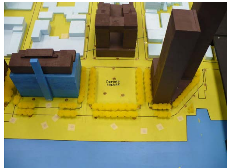
Figure 1: Wind Tunnel Model
