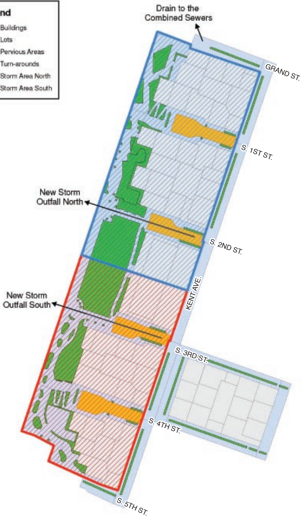
Stormwater Drainage with the Proposed Project
