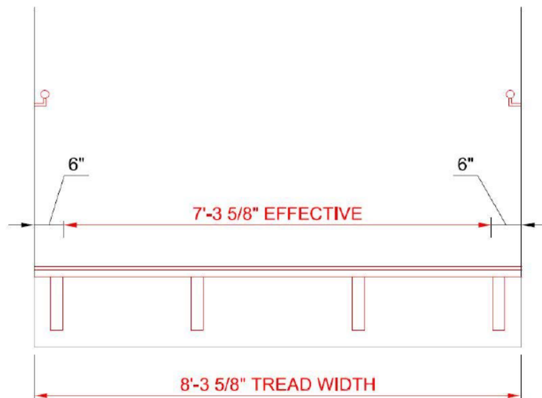
Figure 4: Proposed cross section of stair S1/P1 with multiple stair stringers beneath full width stair treads.
