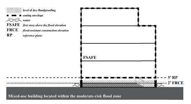
A #zoning lot# located within the #moderate-risk flood zone# has a #flood-resistant construction elevation# (as defined in Section 64-11) of two feet above the lowest grade adjacent to the #building or other structure#. The owner of a #mixed building# that was flooded during Hurricane Sandy, would like to proactively comply with #flood-resistant construction standards# to be better prepared in the event of a future storm. To realize that, the owner decided to elevate the ground
