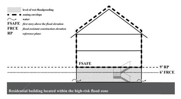
A #zoning lot# located within the #high-risk flood zone# has a #flood-resistant construction elevation# (as defined in Section 64-11) that equates to being located six feet above grade (for illustrative purposes). The owner of a #single-family detached residence# would like to elevate the first habitable floor three feet above the #flood-resistant construction elevation# and wet-floodproof the ground floor up to that same level (nine feet above grade) to account for sea level rise projections.
