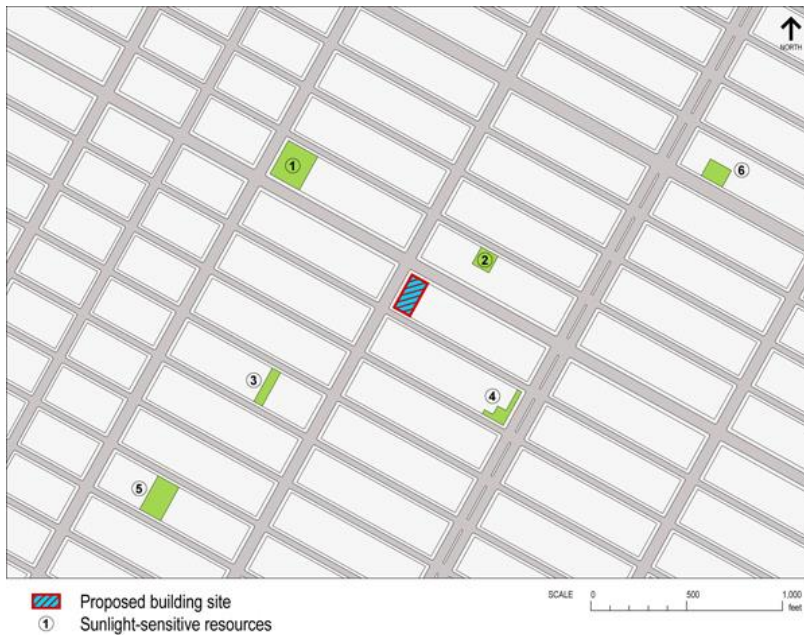
Figure 8-1 shows an example of a base map with the location of a hypothetical building site and a number of sunlight-sensitive resources (labeled 1 through 6) in proximity to the site.
