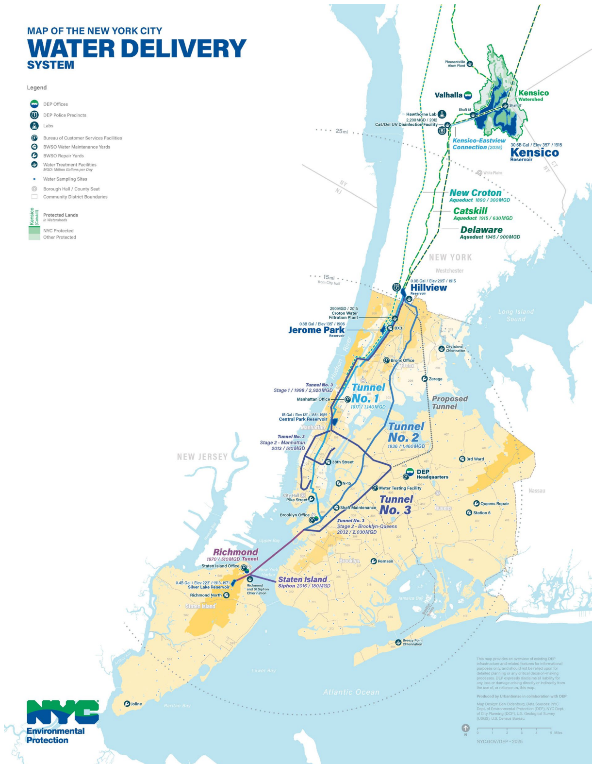
Figure 5-2: New York City Water Conveyance Infrastructure
