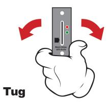
These devices are usually attached with two sided tape and can be discovered by simply tugging on areas where the card must be swiped.
