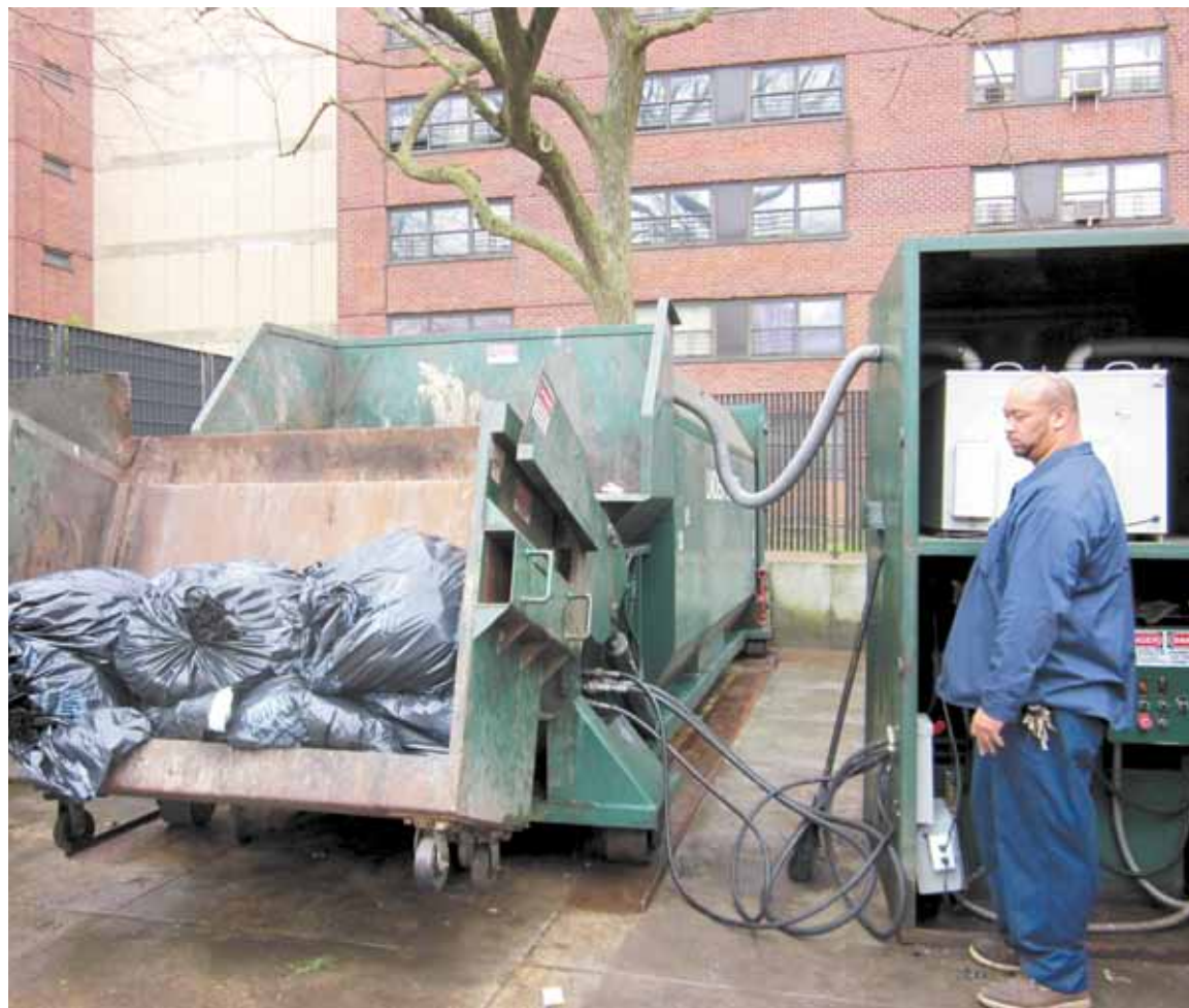
A NYCHA staff member shows how garbage is compacted and deodorized by the compactors at Linden Houses in Brooklyn. Washington Houses (Manhattan) residents were being shown how the process works, because similar compactors will be installed at their development.
