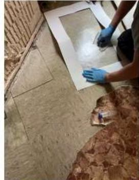
Technician using template to take dust wipe sample. Sample packaged in rigid centrifuge tube. (Building 7 – 131 Ten Evck Walk. Apt 2C)
