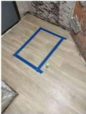
Painters tape used a template to take dust wipe sample. Sample packaged in hard shell container. (Building 2 – 210M W 153<sup>rd</sup> St., Library)
